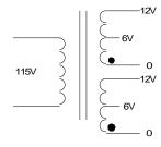
\* Secondaries windings are designed to be connected in series or parallel. Windings are not intended to be used independently.
